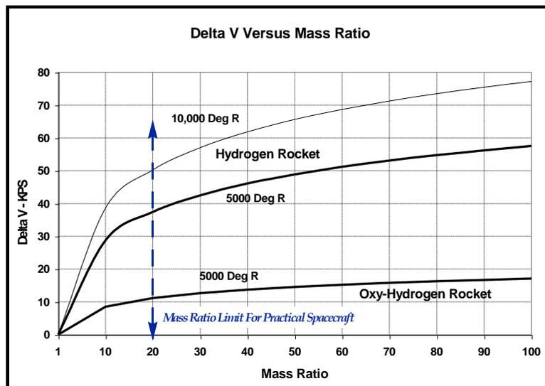
Figure 6: Delta V for Hydrogen Rockets
