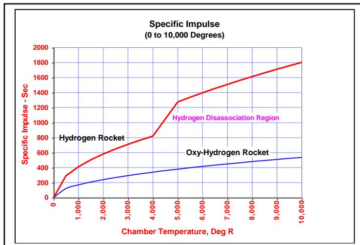
Figure 5: Specific Impulse for Hydrogen Rockets
