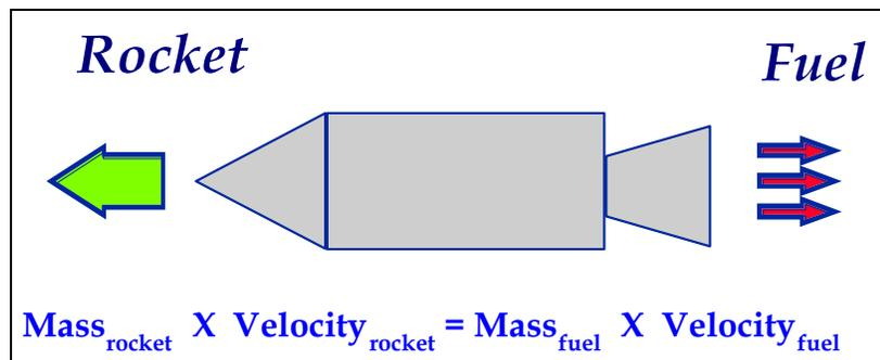
Figure 1: The Rocket Propulsion Principle
