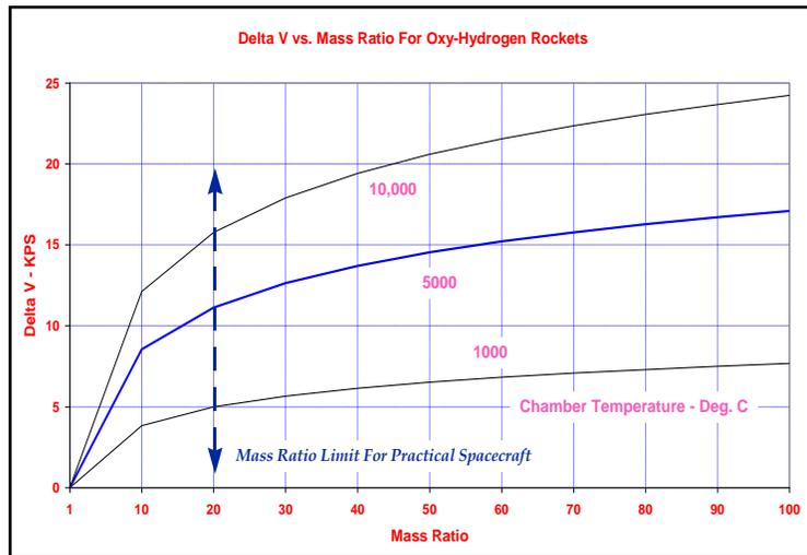
Figure 4: Delta V for Oxy-Hydrogen Rockets
